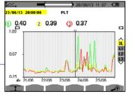
Voltage dips, short outages and long outages (> 10 minutes) were captured. According to the measurements, these disturbances mainly affected L1.
