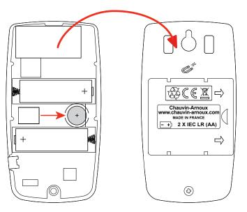
Remove the used button battery by lifting it and replace it with the new batter, respecting the polarity.
