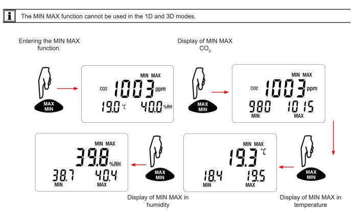
When the **MIN MAX** function is activated, recording of the minimum and of the maximum starts but the display of the three quantities measured makes it possible to continue using the device normally.
