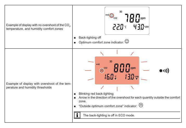
For the **1D** and **3D** modes, if the buzzer is active, it will sound intermittently upon the appearance of the O symbol.
