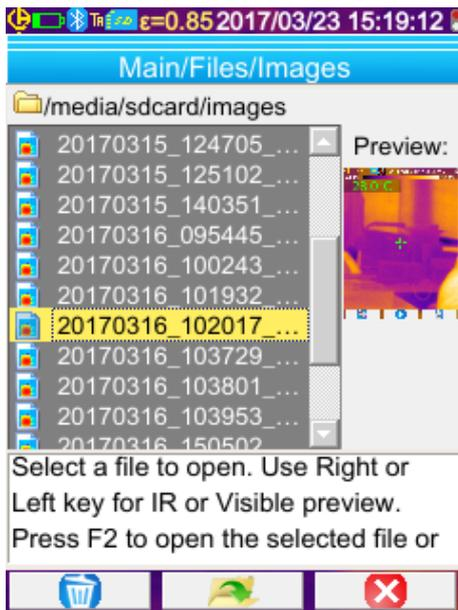
The file manager lists only infrared images generated by the camera bearing a name in the form `yyyymmdd_hhmmssX_IR.PNG`, along with the folders, to allow browsing in the tree of the SD card.
