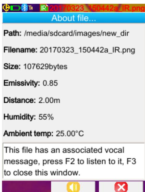
A vocal message is played back using the Bluetooth headset, which must be connected to the camera (see § 6.2.2. [How to connect a headset](#)).
