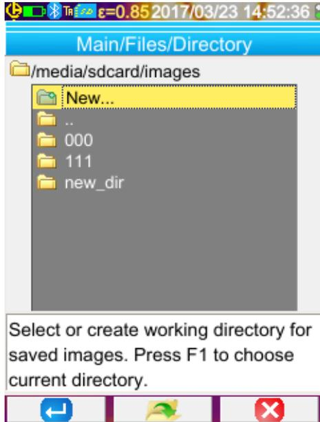
The working directory must be located on the micro SD card, which must be present in the device.
