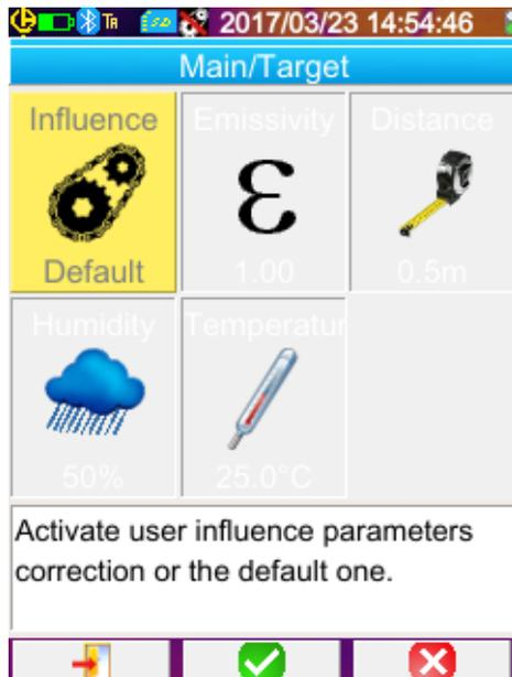
The default compensation for the influencing factors matches the context of calibration of the camera (example: the emissivity is set to 1.00, the distance to 0.5m, the relative humidity to 50%, and the ambient temperature to 25°C).
