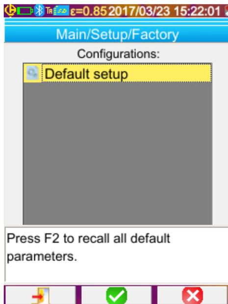
The default setup is one of the predefined configurations proposed in the Main/Setup/Factory menu.
