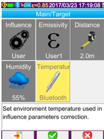
In case of Influence parameters, the measurements replace the user data entered in the Main/Target menu, provided that user influence is selected (see § 3.2.2. [Using the user compensation for the influencing factors](#)).
