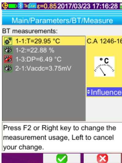
For the measurement to be used as an **influence**, the use "influence" must be assigned to it in the Bluetooth measurements viewing window (Main/Parameters/Bluetooth/Measurements menu):
