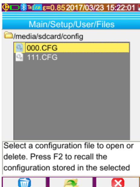
A setup file is recalled from the Main/Setup/User/Files menu, by means of the file manager, which lists all of the configuration files (extension .CFG) found in directory « /media/sdcard/config/ ».
