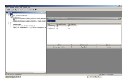
The data are recovered in PAT software. Display of the data in Text mode, in the format « date – time – MIN – AVG – MAX ».
