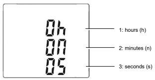
The duration of the metering uses the following format: XXXh (for hours) XXm (for minutes) XXs (for seconds)
