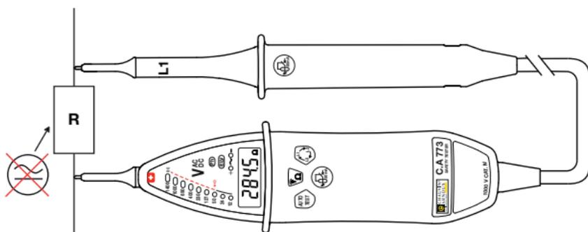
If the device has been idle for more than 10 minutes or if it was set to stand-by mode, run a self-test first, to place it in active stand-by.
