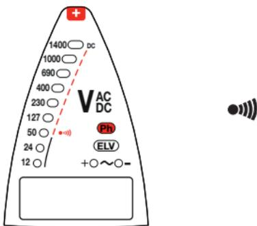
**Note:** The fact that the **Ph** indicator is not flashing does not mean that there is not a hazardous voltage on the connector.
