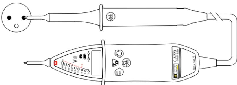
If the test probe is on the phase, the **Ph** (phase) indicator flashes and the device beeps.
