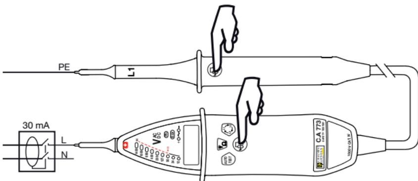
If the voltage measured is between 8 Vrms and 400 Vrms, the test is triggered.
