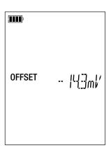
During the calibrations, the offset of a given electrode must not vary more than a little. If you observe a large variation, redo the calibration. If the problem persists, check the buffer solution (in particular the use-by dates) or replace the electrode.
