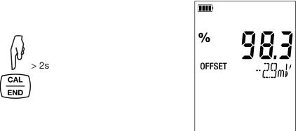
During the calibrations, the slope and offset of a given electrode must not vary more than a little. If you observe a large variation, redo the calibration. If the problem persists, check the buffer solution (in particular the use-by dates) or replace the electrode.
