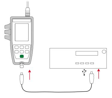
Once the Data Logger Transfer software has been installed, connect the instrument to the PC.
