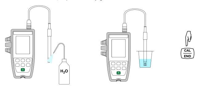
■ Wait for the measurement to stabilize. Once again, the instrument proposes terminating the calibration (by pressing the **END** key) or continuing at a third point (by pressing the **CAL** key).
