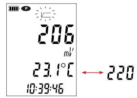
The instrument makes the ORP measurement and indicates its progress.
