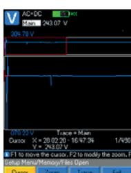
Screenshot of a recording of the variation of a 50 Hz voltage on the ASYC IV.
