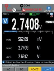
The graphical screen allows you to monitor the voltage drop using the SURV mode in order to recover the time/date-stamped MIN/MAX values.
