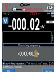
On the multimeter, the minimum acquisition interval programmed is 0.3 s.
