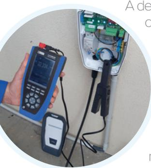
A dedicated function can be used to configure the transformation ratio of the current clamp, with current or voltage output (wide range of current clamps compatible with ASYC IV). Once this ratio has been defined, the multimeter directly displays the current value measured, making it easier to process the results.
