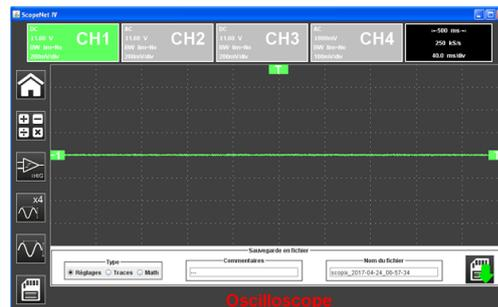
When you have obtained the IP address of the Scopix IV (DHCP or manual) using a browser, type 14.3.250.51/scopenet.html (for example) on your computer → this opens the screen shown opposite.
