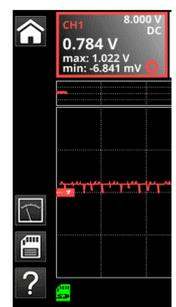
b) Select «logger» mode (Recorder) and calibrate 500 mV/div. fix duration of 10 000 s with resolution of 0.2 s on the on home screen: automatic recorder on files .rec.
