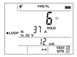
■ The measurement starts automatically. The result is displayed: the loop impedance and the short-circuit current (Ik). Press the **TEST** key to return to voltage measurement.
