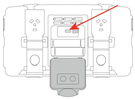
■ Simultaneously press the button and the **MEM** key (for the C.A 6133) or the key (for the C.A 6131). The instrument displays **SOFt UPd**.
