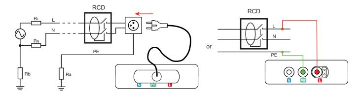
The instrument first of all checks that the voltage between the L and PE terminals is correct. If it is, the  $\frac{1}{2}$  symbol lights steadily. If not, the symbol blinks and it is not possible to make a test. If  $U_{\text{LPE}} < 90 \text{ V}$ , the instrument displays  $U_{\text{LPE}}$  and  $U_{\text{NPE in}}$  alternation.
