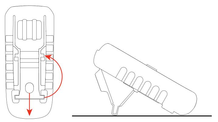
The stand can also be used to hook the instrument on a door.
