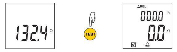
At each new measurement, the instrument indicates the difference between the new reading and the reference measurement, along with the difference in %.
