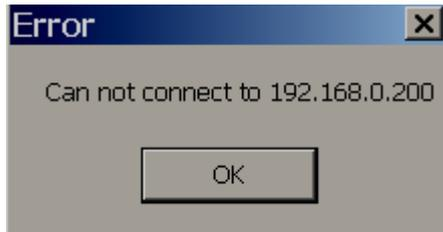
If CPS Touch is disconnected when CPS Remote Viewer session is running, it may show "Communication error" message in some objects like Text box etc.. no special alert messages are displayed in CPS Remote Viewer
