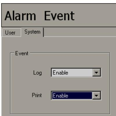
Log= Enable, it means, event will be logged to internal memory/SD card if configured
