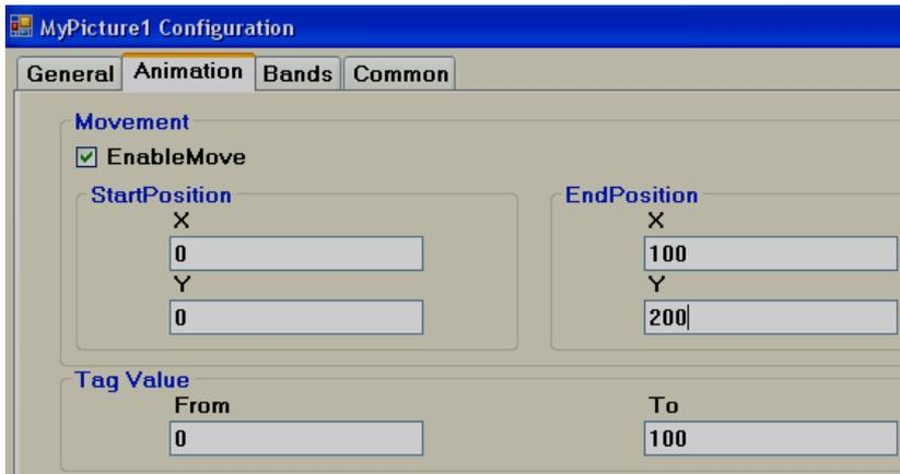
**Movement:** Select Enable/Move and then, enter X and Y start and end positions in pixels.
