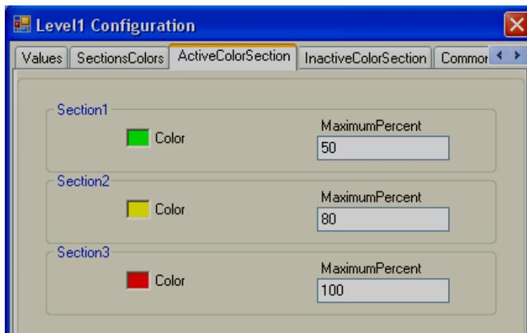
**Active Color Section:** Define Active color for process value band. For example: If process value range is 0-100, set different bands in % for process value, define colors to appear with in level Bar graph in Run Time.
