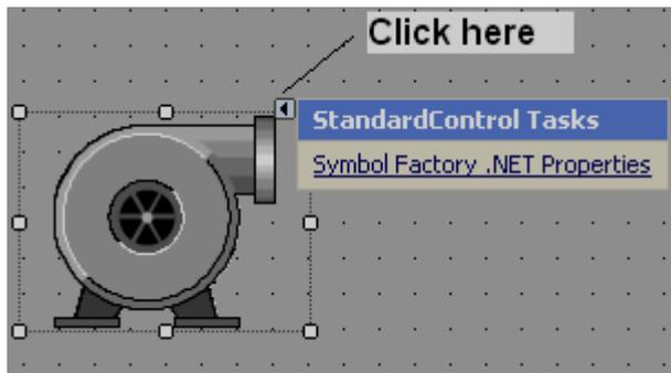
Drag and drop symbol factory component into screen.
