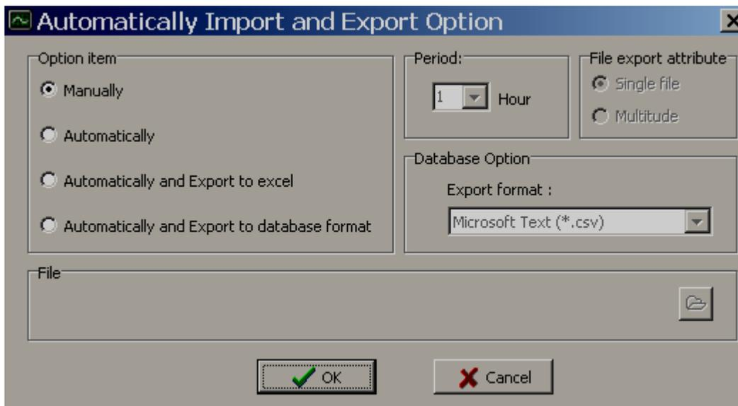
**Manually:** Select this option if it is required to import historical data and alarms manually from device to PC
