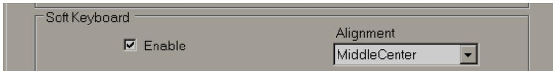
**Soft keyboard:** If enabled, then, it is possible to control the keypad appearance in run time. For example, if alignment is selected as Middle center, then, when keypad appears in run time, it will be located to Middle center in screen
