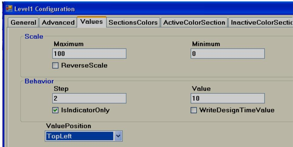
**Maximum:** This is maximum range of process value (Analog input Type Tag)
