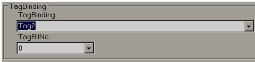
In above fig, Tag2 is analog type (4 byte), so, TagBitNo combo box will appear for selection of required bit with in 32 bits (0 to 31).
