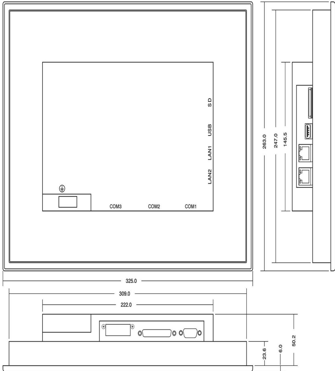
Note: All dimensions are in mm. Tolerance +/- 1 mm
