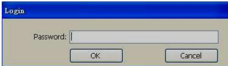
9. Now, you have to enter Password set at Control Center. If password match with password set at CPS Touch Control center, CPS Touch screen will be transferred to PC. Otherwise, it will give message about incorrect password
