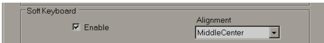
**Soft keyboard:** If enabled, then, it is possible to control the keypad appearance in run time. For example, if alignment is selected as Middle center, then, when keypad appears in run time, it will be located to Middle center in screen
