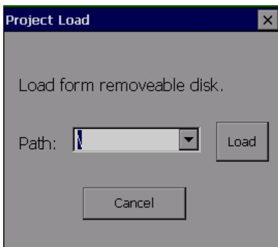
Press “Down” arrow and select the path, if folders are available in USB stick. Then, press on “Load” button near the combo box. If project file is available in selected path, then, it will transfer from USB stick to CPS Touch.
