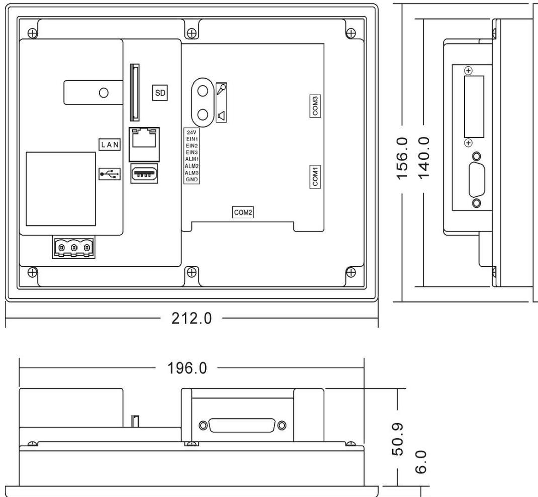
Note: All dimensions are in mm. Tolerance +/- 1 mm
