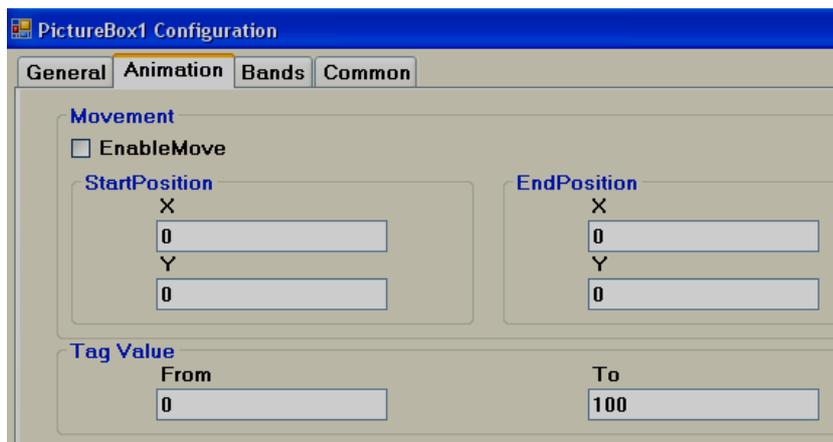
**Movement:** Select Enable Move if it is required to move picture in Run time from Location 1 to Location 2 based on tag Value. Start and End coordinates for X and Y needs to be configured in Design time and Picture moves in Run time based on Tag value.
