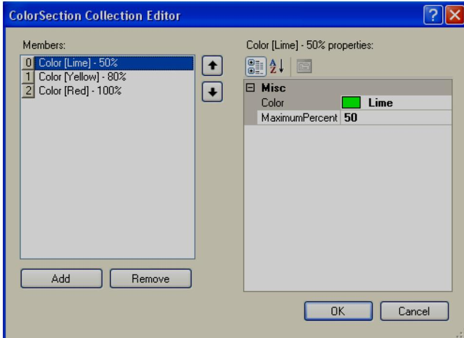
**Inactive Color Section:** Define Inactive color for process value bands same as above. Generally light colors are selected for Inactive colors and Dark colors with more contrast is selected for Active colors, then users/operators will be able to differentiate between active and inactive colors clearly.
