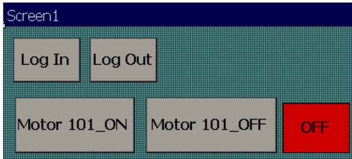
Use Log In, Log Out events with buttons first. Now, when operator Log in, it will record event in the Historical alarm box, it shows which operator log in to CPS Touch
