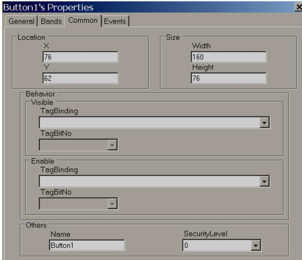
**Security control:** Define security level for button. It allows user to operate the button only when operator security level is equal to or more than security level defined here.
