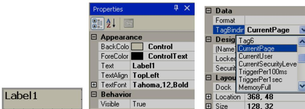
**Current Page:** Display current page number. It is Analog type system tag and support Read/Write functionality
