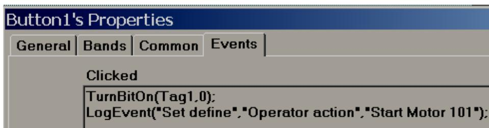
When operator press Motor 101\_ON button, first it turn bit ON, then, it will log in message “Operator action” at “Name” and “Start Motor 101” at “Message” column in historical alarm box.
