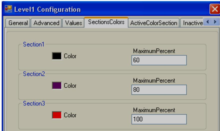
**Sections colors:** It is configure bands for the sections to show different colors for Labels and Ticks in Level graph.
