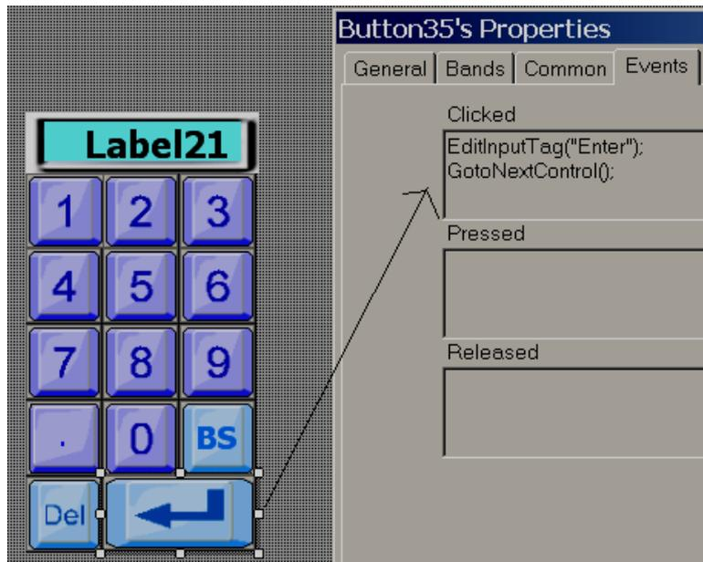
For example, in this application, if cursor is first located at Textbox1 in run time, then, if operator enter value 123 from keypad and press “Enter” softkey, the value available at InputTag buffer will be moved to Textbox1 and then cursor will move to next Textbox as per Tab index value
