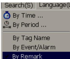
Alternatively, near the task bar at bottom area of the screen, click on “Seek by Remark”
