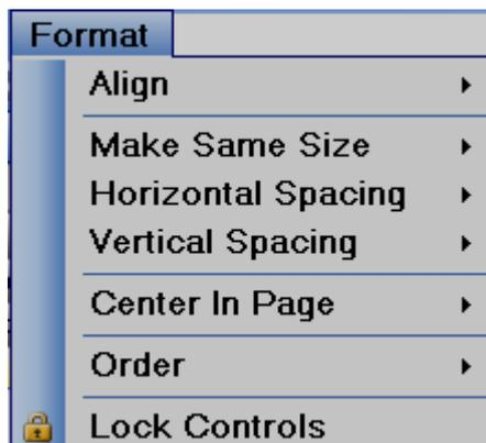
**Align:** It is to align selected components, objects etc. for adjusting their position precisely in screen layout. Available options for selection are Center, Right, Left, Top, middle & Bottom.
