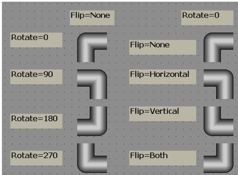
**Rotate:** Rotate symbol to any predefined direction in specific band at Run time. Available options include  $0^{\circ}$ ,  $90^{\circ}$ ,  $180^{\circ}$  and  $270^{\circ}$
