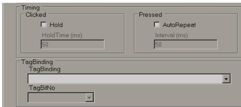
**Timing:** This is an advanced feature and used to make sure operator action is properly received by PLC when PLC scan time is large.
