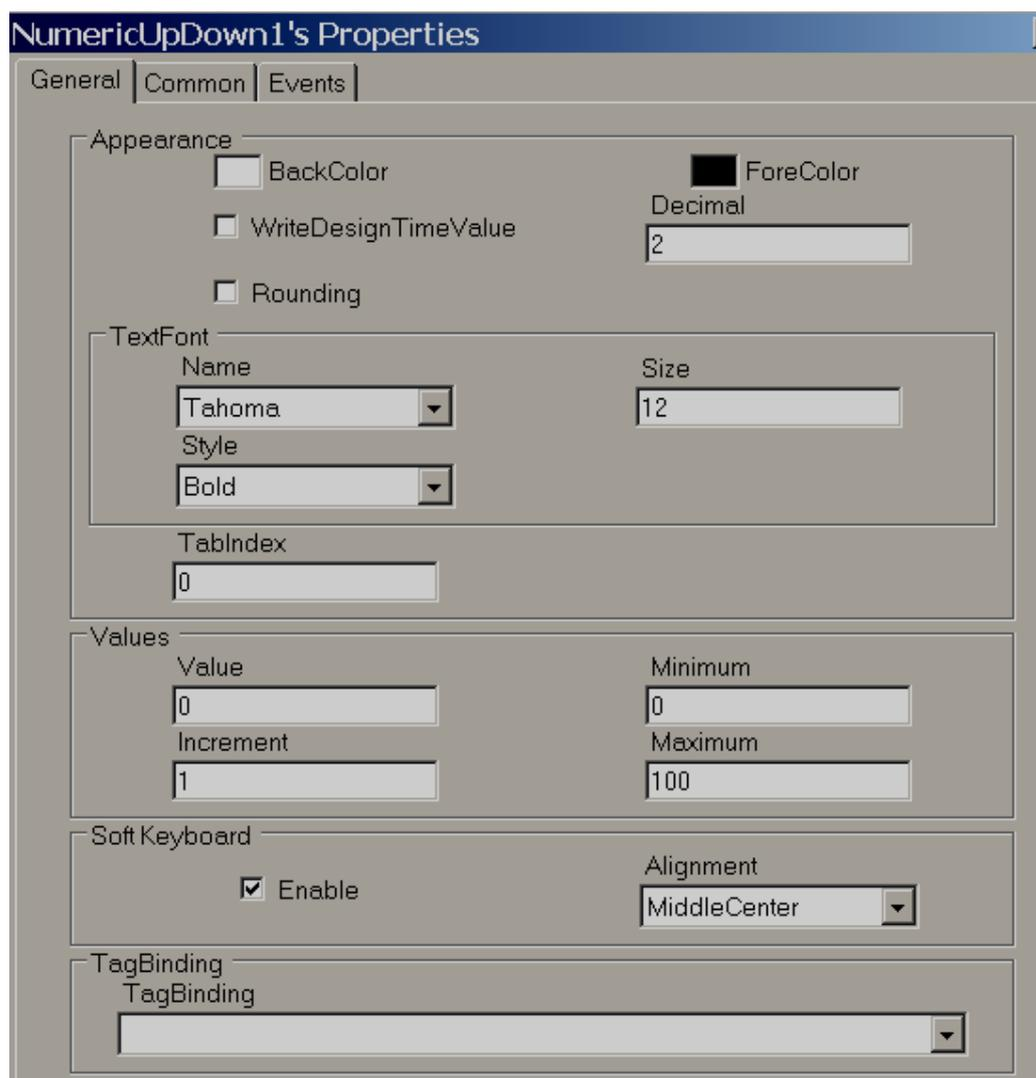
Increment: Select the value to be incremented/ decremented each time when up/down arrow is pressed in Run time.
