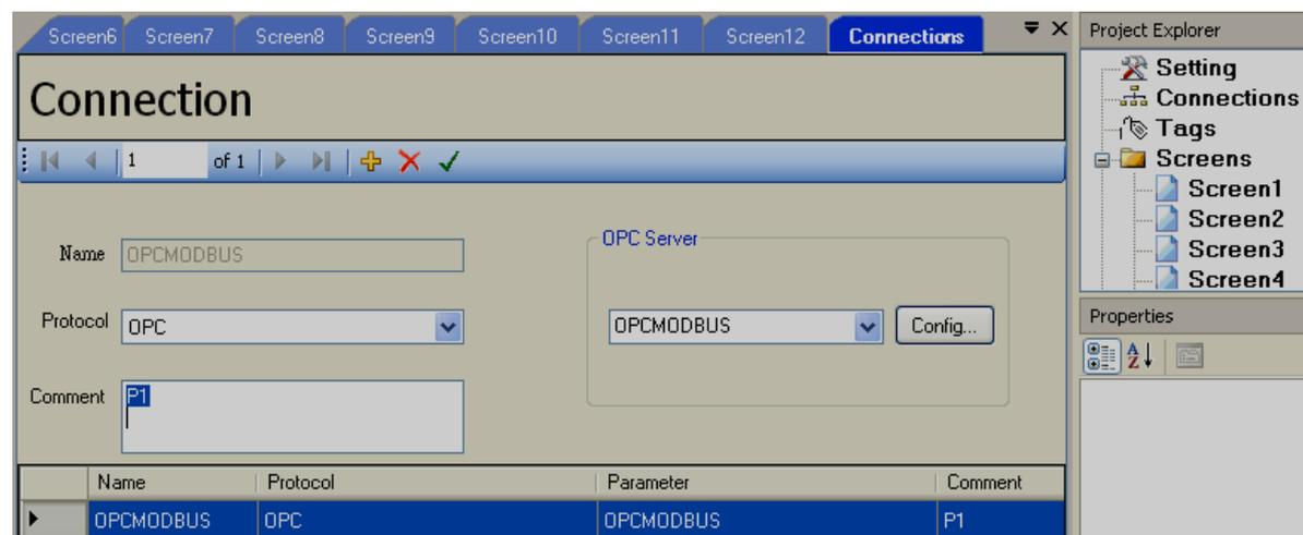
Step-3: Connect IO module to PC via RS485/RS232 converter, assume it is COM1 in PC. Now, PC is being used instead of CPS Touch for testing purpose. PC is Modbus RTU Master and IO module is Modbus RTU slave.
