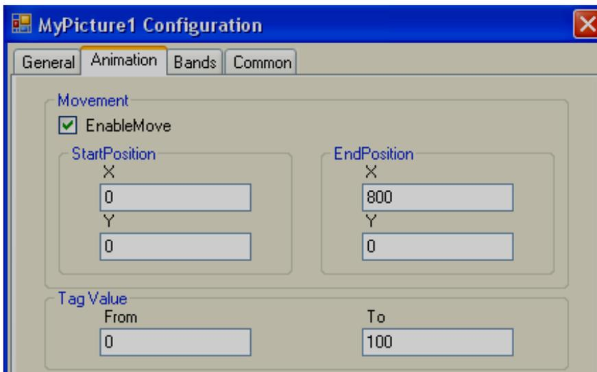
To move symbol from Left to Right, set start and end Positions for X coordinate in pixels and there is no need to set Y coordinates.
