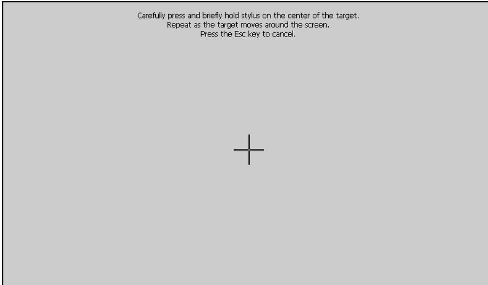
Initially target will be at center. Carefully press and briefly hold stylus on the center of the target. Repeat this procedure as target moves around all the 4 corners.
