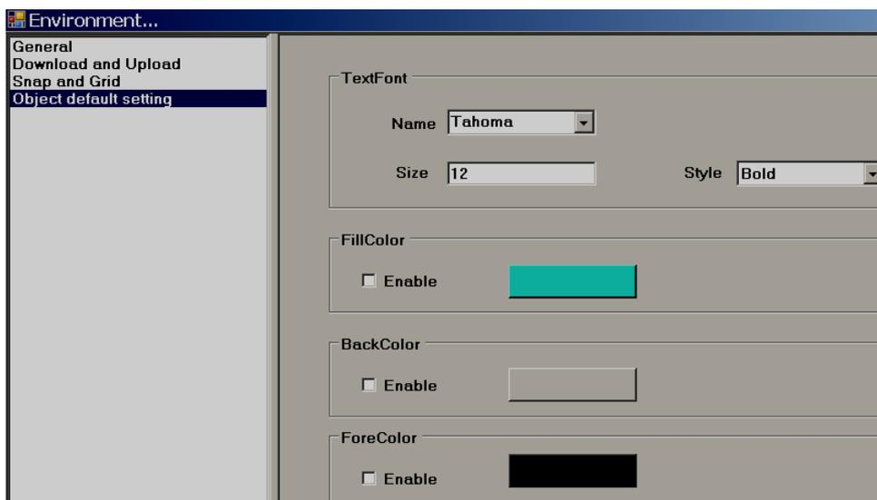
**Object:** Define default font size, Fill color, Back color and Fore color for the properties of most of the objects like label, Check box, Rectangle, Ellipse, Pie, Table, Dial, Level, Meter, Slider, Thermometer etc.
