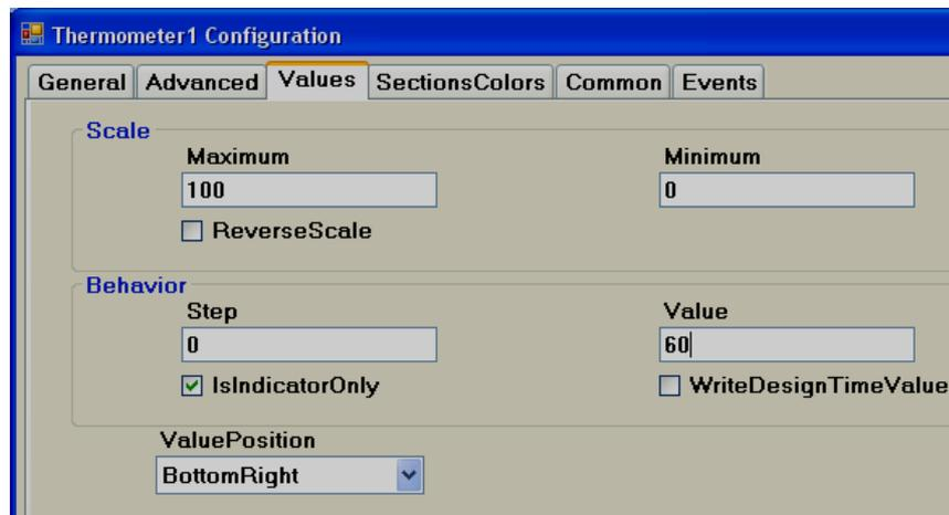
**Maximum:** This is maximum range of Set point (Analog Tag, Normally Analog input, 20 mA, 10V DC etc.)
