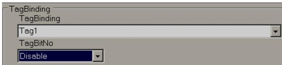
If Tag1 is Analog Type (32 bit), it is also possible to show different display based on individual bits. By default, it is disabled. You can select the bit from the combo box and then configure band editor as per project requirements.
