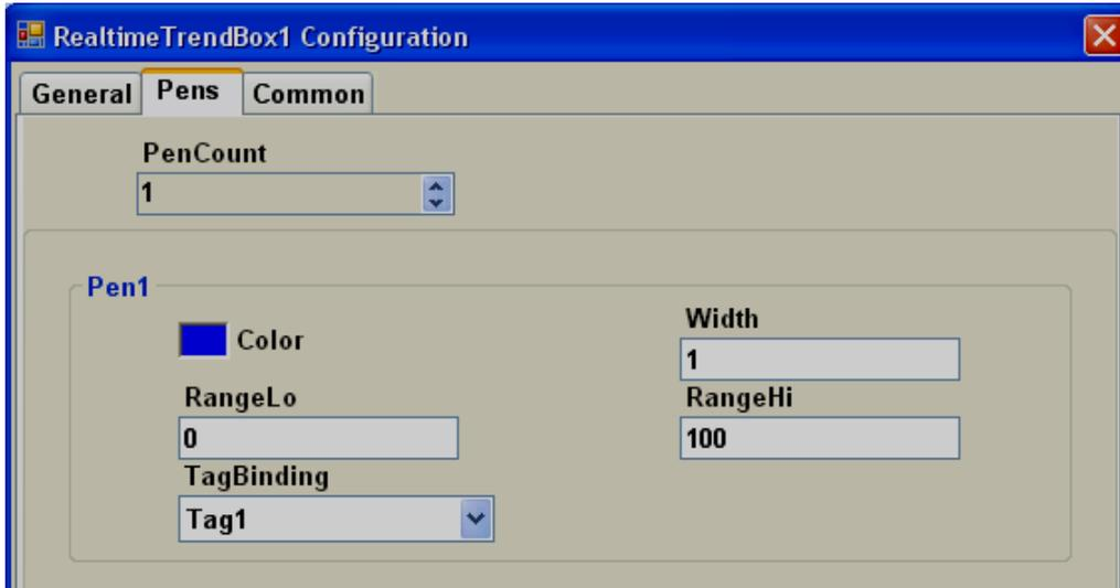
**Pens:** It is to configure required pens to view on specific Real time trend object in Run time. Use Up button on Pen count to add pens and then configure all the properties for specific pen say Color, Width, Range, Tag binding etc.
