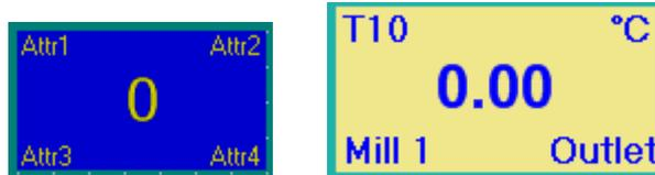
Every Digital Box normally used with **Analog** Tag to display process values like Temperature, Pressure, Flow etc., It also allows 4 different labels as attributes for displaying tag related information.
