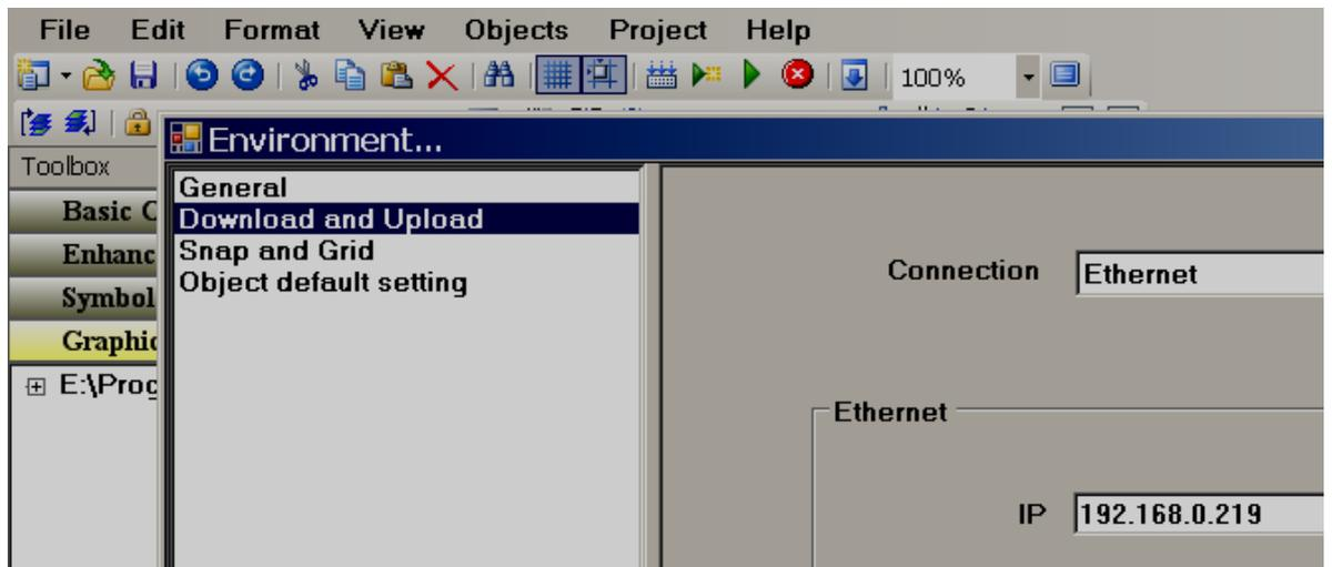
First enter IP address of CPS Touch at Environment settings in CPS Studio as shown above, then, try to update firmware from PC to CPS Touch via Ethernet
