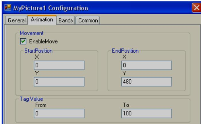
**Ex: CPS7, Screen Resolution = 800 X 480, Horizontal installation, Width=800, Height=480. Move symbol from Left Top to Right Bottom in screen in angle at Run time when tag value changes from 0 to 100**
