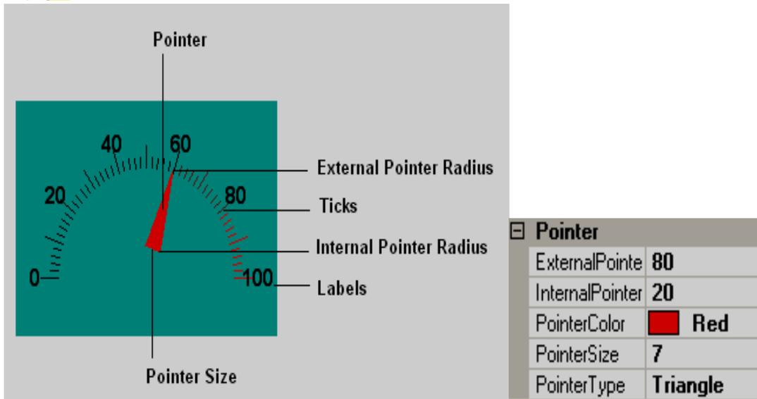
**External Pointer Radius:** It is to set external pointer Radius, define end position.
