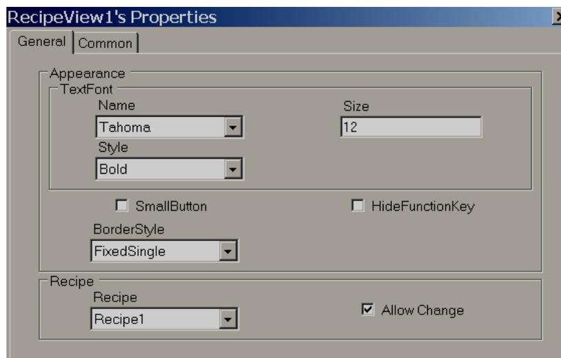
**SmallButton** Select this option to change all soft buttons to small size and this is most useful while using Recipe object in CPS4
