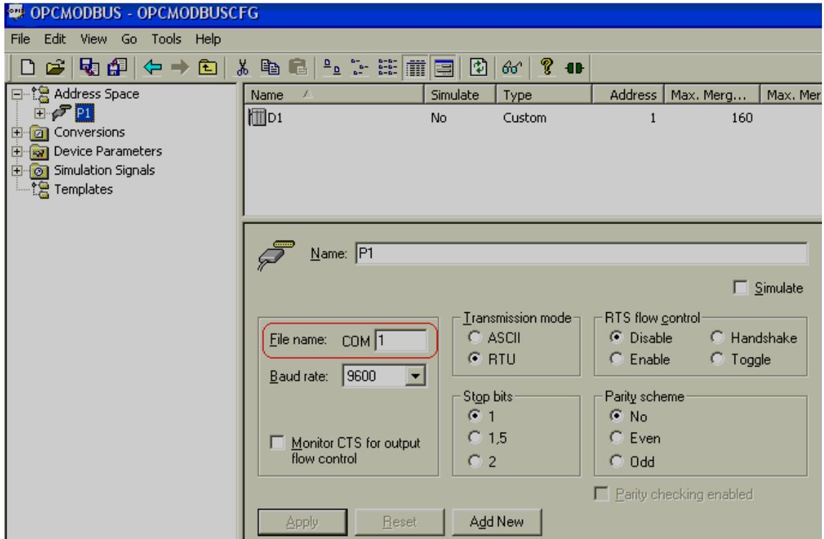
Step-4: Select COM port properly. This is COM port number in PC to which slave device is connected.
