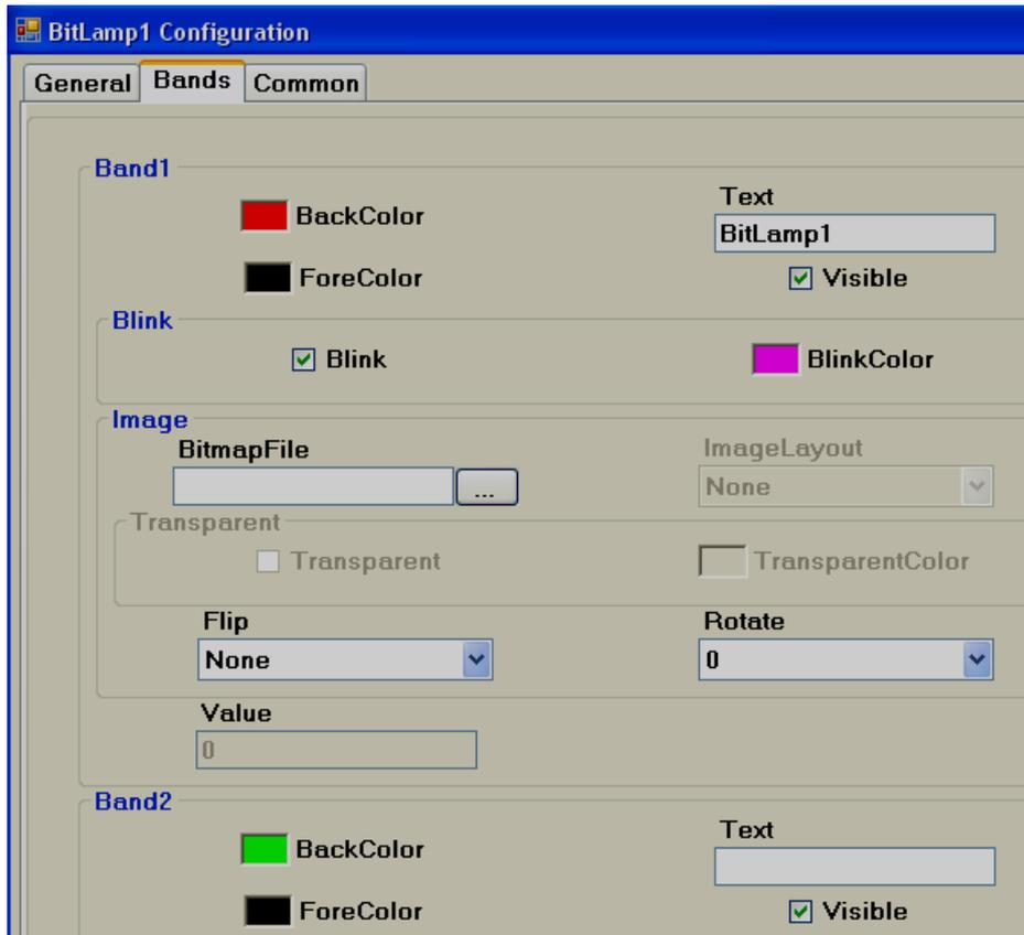
**Bitmap file:** Select the image to be displayed when tag value reaches this band in run time.
