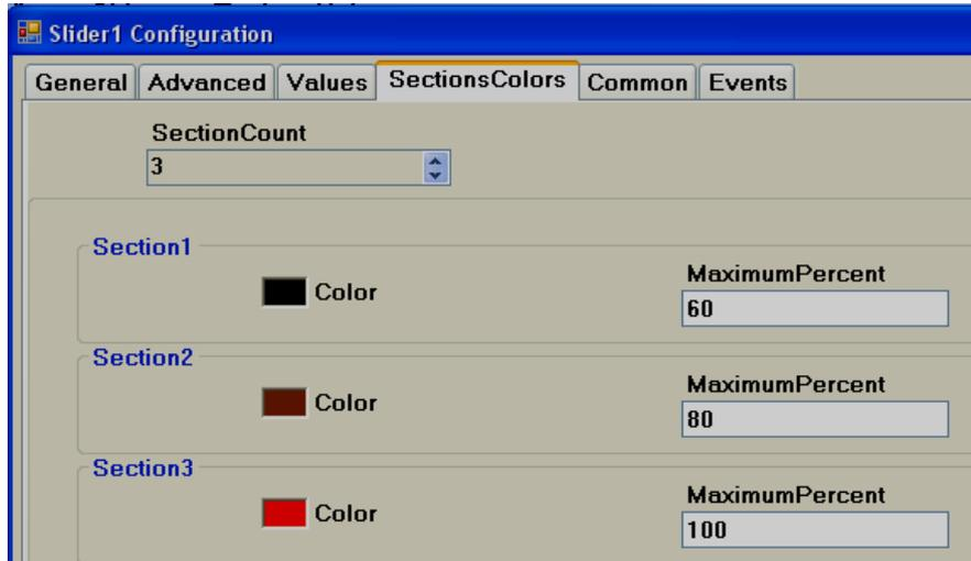
**Sections colors:** It is configure bands for the sections to show different colors for Labels and Ticks in Slider.
