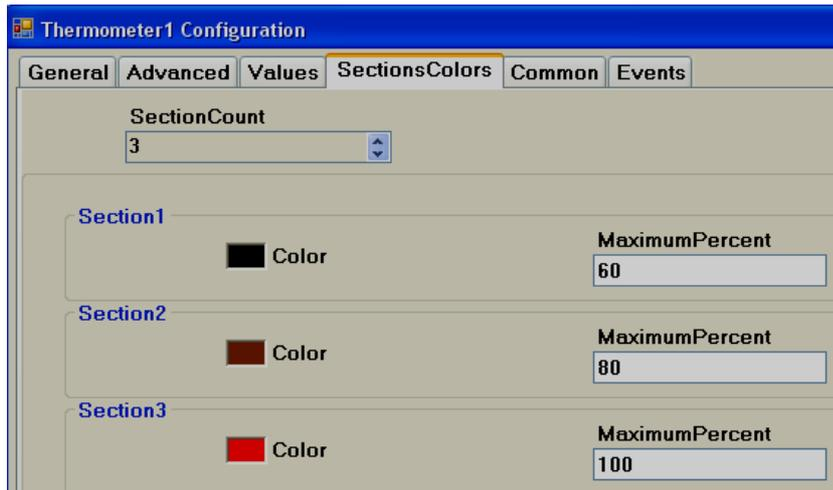
**Section Colors:** Define bands to display Ticks and Label color accordingly based on value of tag in Run time.
