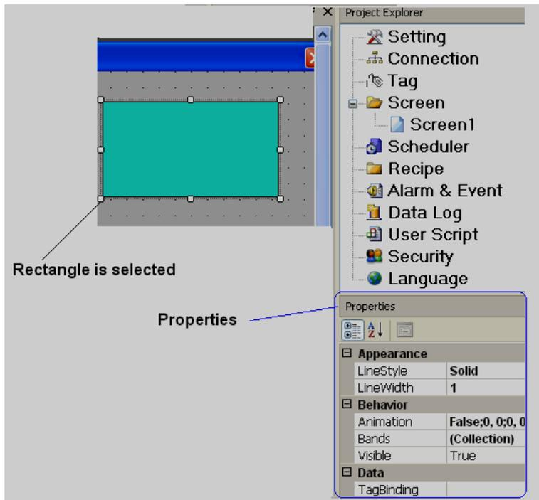
In above example, rectangle is drawn and once it is selected, then right side bottom corner, it shows all the properties for this specific rectangle if properties are checked in view at Menu bar. It is possible to modify properties of rectangle from property grid. Alternatively, double click on Rectangle and enter the same at Graphical wizard.
