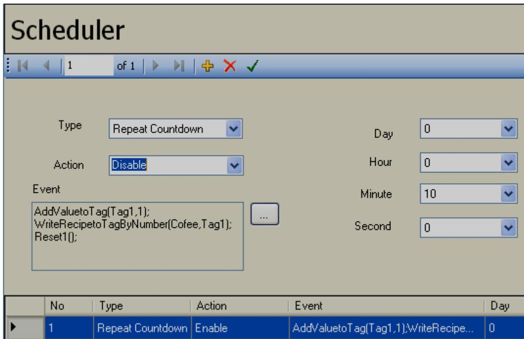
3. Select the Recipe and Data record number to be written from CPS Touch to PLC by using function “WriteRecipetoTagByNumber(Cofee, Tag1)”
