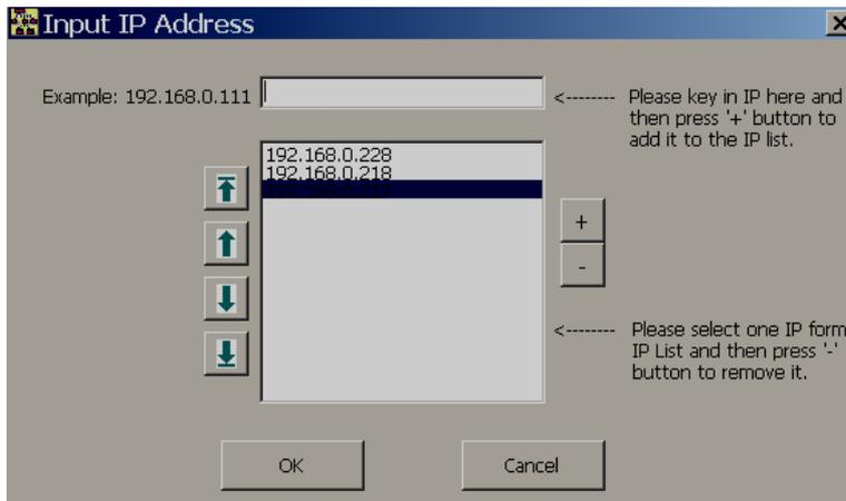
Select IP address of CPS Touch to be removed, then click at soft button
