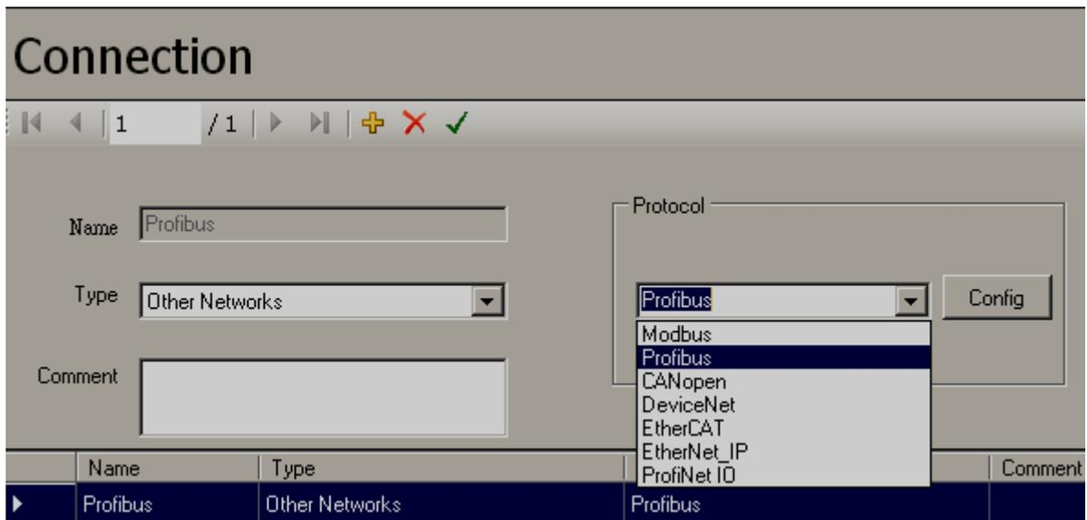
Note: Select Modbus from “Other networks” only for old projects using plug in Network option module for Modbus RTU Slave function. CPS Studio V1.10 onwards, Modbus RTU and TCP slave drivers added onboard using standard Serial & Ethernet ports, no special plug in module required
