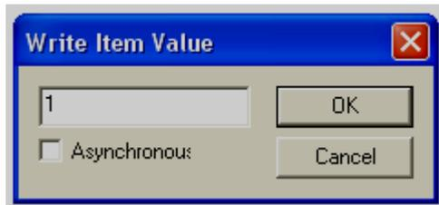
Write value 1 to switch on digital output
